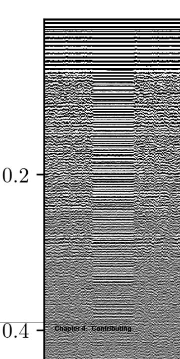
We still probably have some noise coming in horizontally (e.g. long-wavelength changes in return power due to our batteries draining in the radar controller). To remove this, we can remove something akin to the average trace.
