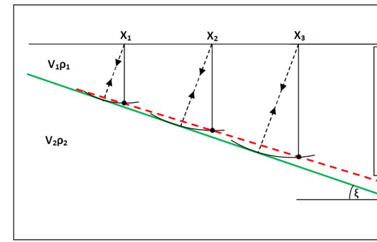
The migration problem is illustrated in the image above. Dipping reflectors are imaged by an off-nadir ('apparent') reflection. The ray path of the apparent reflection is not the same as the depth of the reflector directly below the source. The *migrator's equation* is a simple analytic way to adjust the angle of a dipping reflector,
