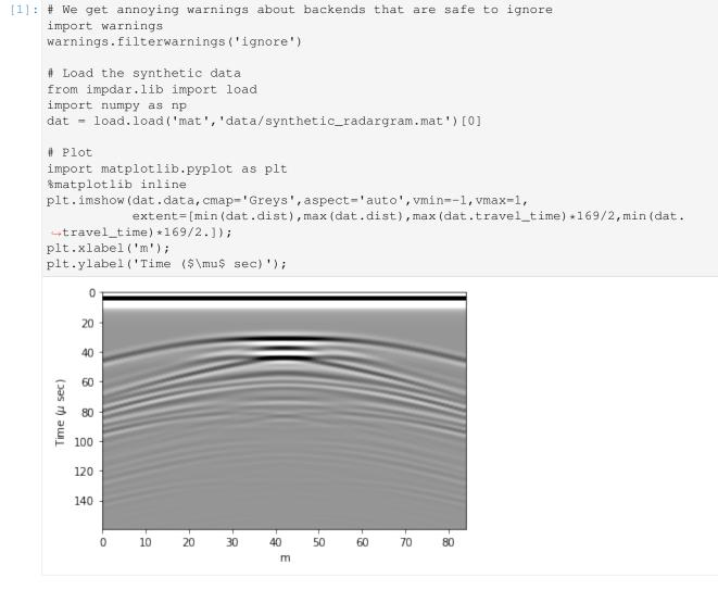
This synthetic image illustrates why we need to migrate. There are large hyperbola that extend away from the actual location of the box in both horizontal directions. These hyperbola, or diffraction curves, do not accurately represent the subsurface stratigraphy, they are only a result of imaging the box from the side as an off-nadir reflector.
