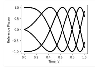
The ImpDAR function, apres\_range, uses the reference phasor shown above to convert from the elapsed time to a range measurement. As explaned by Brennan et al. (2013) section 3, the FFT-processed waveform is weighted by the phase conjugate of the reference phasor to do the pulse compression. After executing this function, the data are more interpretable.
