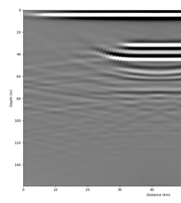
Stolt migration is great in places where the velocity is known to be constant. It is quite a bit faster than the other routines. Here though, we need to be careful about migrating power in from the edges of the domain, as can be seen in the lower corners above. For this reason, we apply a linear taper to the data so that the Fast Fourier Transform has
