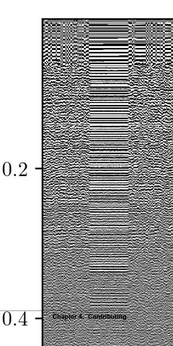
Since layer slopes are small, we have lots of extraneous data. We can restack to reduce noise a bit more and reduce filesize.
