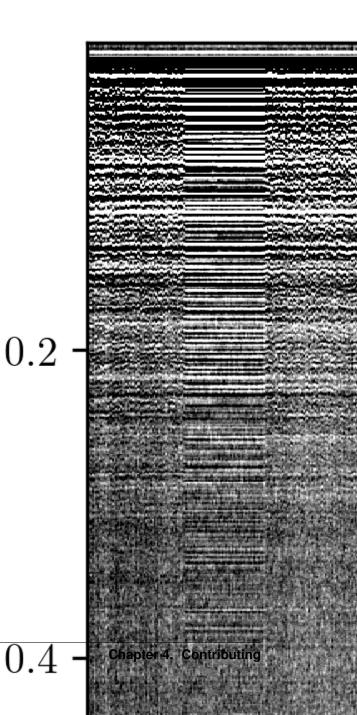
First, lets do some vertical filtering. As before, we will vertically bandpass with a 5th-order forward-backward Butterworth filter from 200 to 600 MHz.
