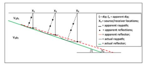
The migration problem is illustrated in the image above. Dipping reflectors are imaged by an off-nadir ('apparent') reflection. The ray path of the apparent reflection is not the same as the depth of the reflector directly below the source. The migrator's equation is a simple analytic way to adjust the angle of a dipping reflector,
