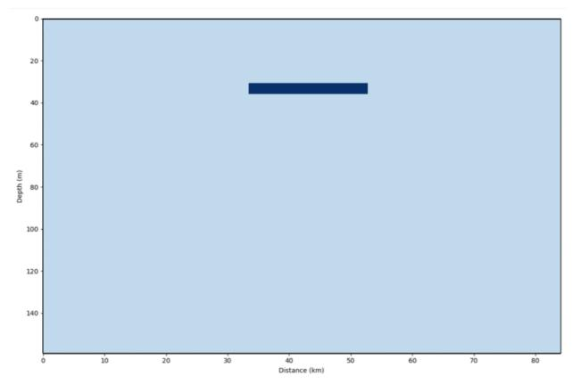
Loading this domain into gprmax (a finite-difference time-domain modeling software), we simulate a common-offset radar survey over the box with the output as a synthetic radargram. The source is a 3-MHz wave from a Hertzian Dipole antenna. Source-receiver antenna separation is 40 m, and the step size between traces is 4 m.
