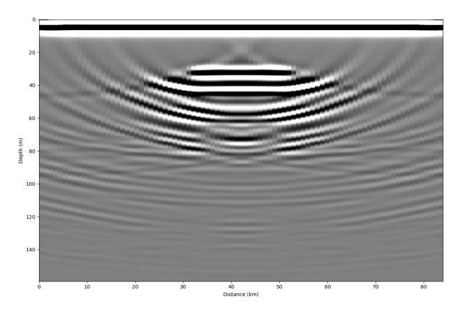
Now we can see the box in its original location (i.e. ~30-55 km lateral distance and ~30 m depth). This method seems to work, but it is slow (even for this small synthetic dataset) and it 'over migrates' through much of the domain as can be seen by the upward facing hyperbola ('smileys') around the edges and below the box.
