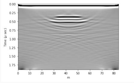
Stolt migration is great in places where the velocity is known to be constant. It is quite a bit faster than the other routines. Here though, we need to be careful about migrating power in from the edges of the domain, as can be seen in the lower corners above. For this reason, we apply a linear taper to the data so that the Fast Fourier Transform being used does not instantaneously switch from data to zeros around the edges.
