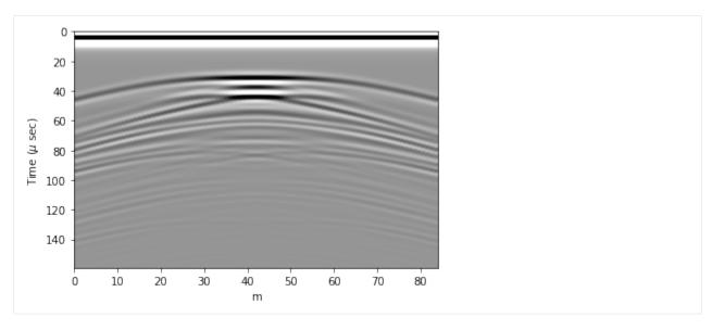
This synthetic image illustrates why we need to migrate. There are large hyperbola that extend away from the actual location of the box in both horizontal directions. These hyperbola, or diffraction curves, do not accurately represent the subsurface stratigraphy, they are only a result of imaging the box from the side as an off-nadir reflector.
