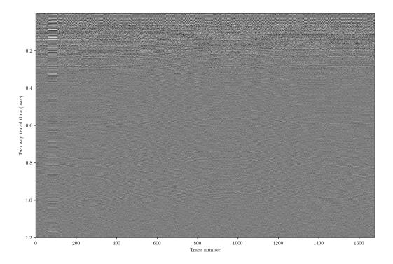
Since layer slopes are small, we have lots of extraneous data. We can restack to reduce noise a bit more and reduce filesize.
