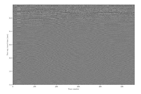
Now we want to look at this in terms of depth. We are going to do this with a constant vertical velocity. This particular data was collected with GSSI radar with a single transmit/receive antenna, so there is no need to do any geometric correction for the triangular pattern of transmit/receive that we would get with spatially separated antennas (like many HF systems have).
