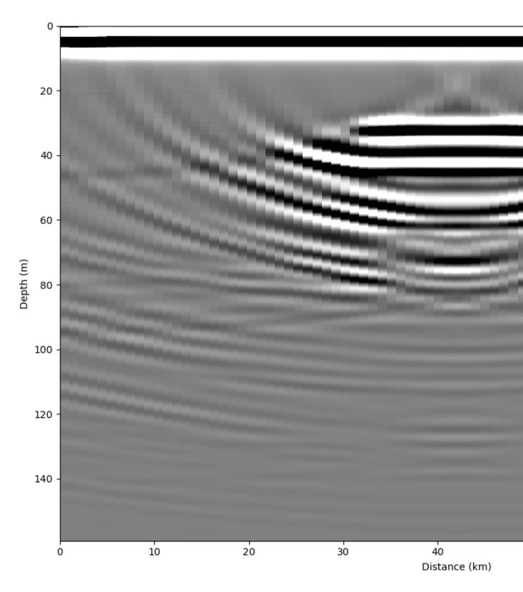
Now we can see the box in its original location (i.e. ~30-55 km lateral distance and ~30 m depth). This method seems to work, but it is slow (even for this small synthetic dataset) and it 'over migrates' through much of the domain as can be seen by the upward facing hyperbola ('smileys') around the edges and below the box.
