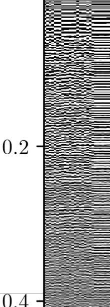
Now we want to look at this in terms of depth. We are going to do this with a constant vertical velocity. This particular data was collected with GSSI radar with a single transmit/receive antenna, so there is no need to do any geometric correction for the triangular pattern of transmit/receive that we would get with spatially separated antennas (like many HF systems have).
