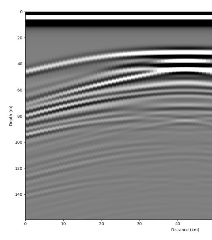
This synthetic image illustrates why we need to migrate. There are large hyperbolae that extend away from the actual location of the box in both horizontal directions. These hyperbola, or diffraction curves, do not accurately represent the subsurface stratigraphy, they are only a result of imaging the box from the side as an off-nadir reflector.
