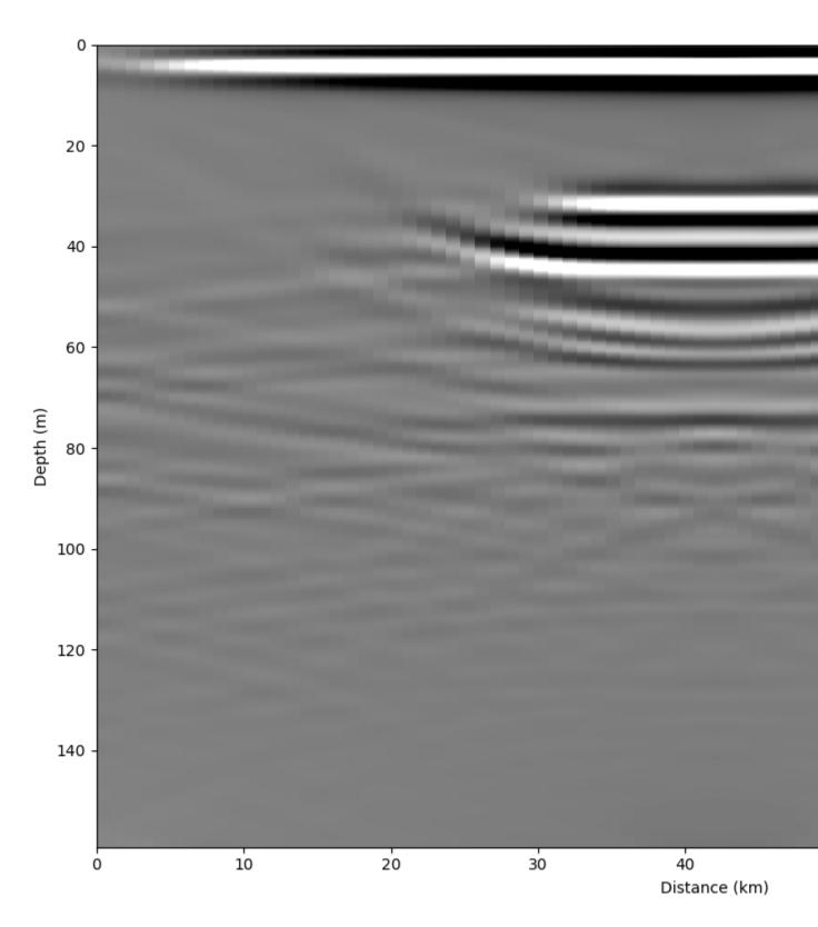
Stolt migration is great in places where the velocity is known to be constant. It is quite a bit faster than the other routines. Here though, we need to be careful about migrating power in from the edges of the domain, as can be seen in the lower corners above. For this reason, we apply a linear taper to the data so that the Fast Fourier Transform has
