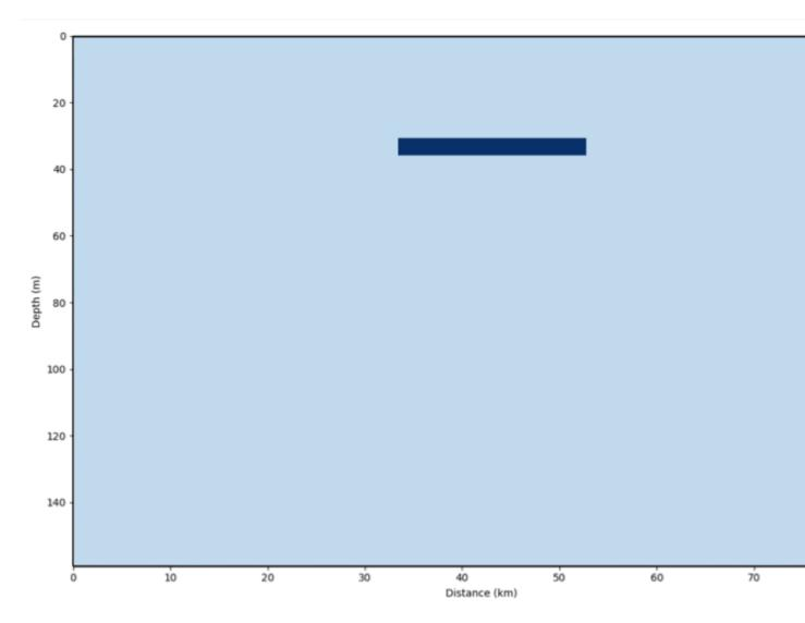
Loading this domain into gprmax (a finite-difference time-domain modeling software), we simulate a common-offset radar survey over the box with the output as a synthetic radargram. The source is a 3-MHz wave from a Hertzian Dipole antenna. Source-receiver antenna separation is 40 m, and the step size between traces is 4 m.
