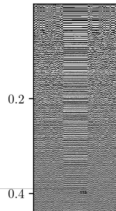
Since layer slopes are small, we have lots of extraneous data. We can restack to reduce noise a bit more and reduce filesize.
