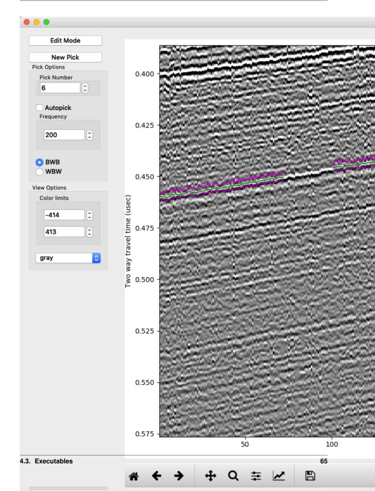
We can also go back and edit a previous pick, moving it up, say. We can also delete picks in the middle of a profile by left clicking at the right edge of the span we are deleting, then right click at the left edge.
