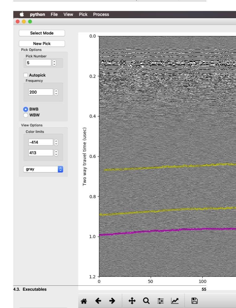
In this profile, I've picked some layers already. The active pick is highlighted in magenta (or rather the top and bottom of the packet are in magenta, and the middle of the packet is green, but the middle is not visible at this zoom). Other picks are in yellow, surrounding a blue central peak. On the left side are most of the controls for when do the picking. We'll go through the buttons on the left, from top to bottom, to get an idea of how picking proceeds.
