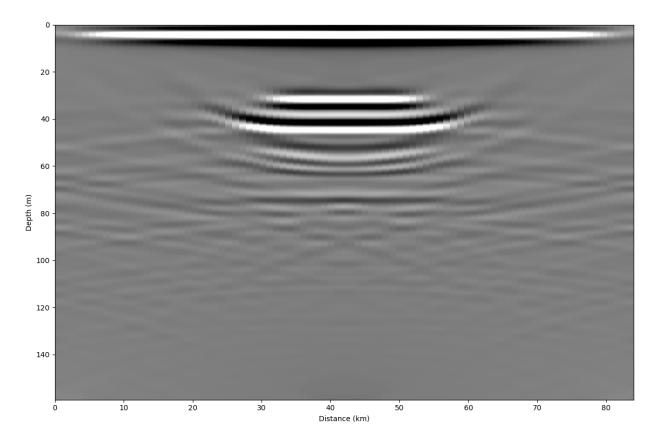
Stolt migration is great in places where the velocity is known to be constant. It is quite a bit faster than the other routines. Here though, we need to be careful about migrating power in from the edges of the domain, as can be seen in the lower corners above. For this reason, we apply a linear taper to the data so that the Fast Fourier Transform has a smooth transition from data to the zeros that it fills in around the edges.
