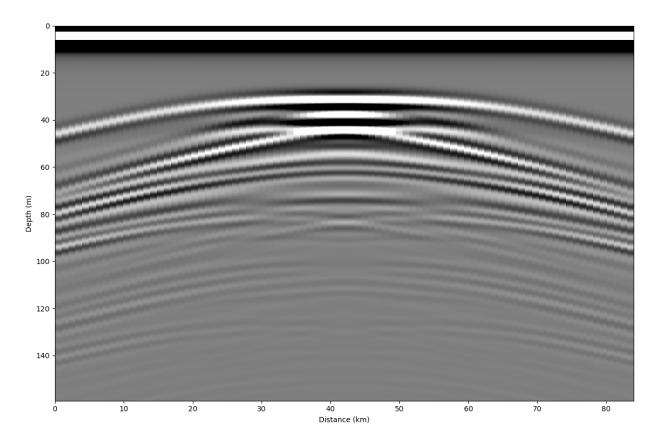
This synthetic image illustrates why we need to migrate. There are large hyperbolae that extend away from the actual location of the box in both horizontal directions. These hyperbola, or diffraction curves, do not accurately represent the subsurface stratigraphy, they are only a result of imaging the box from the side as an off-nadir reflector.
