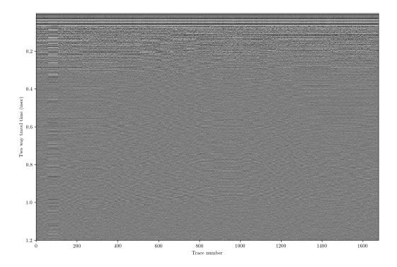
We still probably have some noise coming in horizontally (e.g. long-wavelength changes in return power due to our batteries draining in the radar controller). To remove this, we can remove something akin to the average trace.
