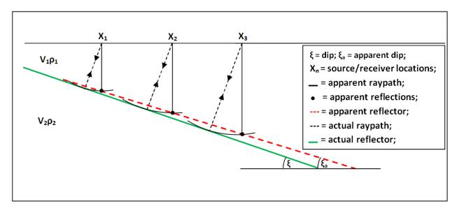
The migration problem is illustrated in the image above. Dipping reflectors are imaged by an off-nadir ('apparent') reflection. The ray path of the apparent reflection is not the same as the depth of the reflector directly below the source. The *migrator's equation* is a simple analytic way to adjust the angle of a dipping reflector,
