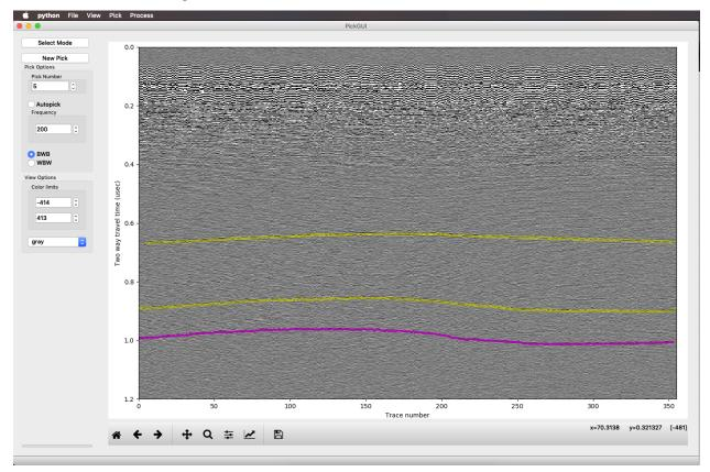
In this profile, I've picked some layers already. The active pick is highlighted in magenta (or rather the top and bottom of the packet are in magenta, and the middle of the packet is green, but the middle is not visible at this zoom). Other picks are in yellow, surrounding a blue central peak. On the left side are most of the controls for when do the picking. We'll go through the buttons on the left, from top to bottom, to get an idea of how picking proceeds.
