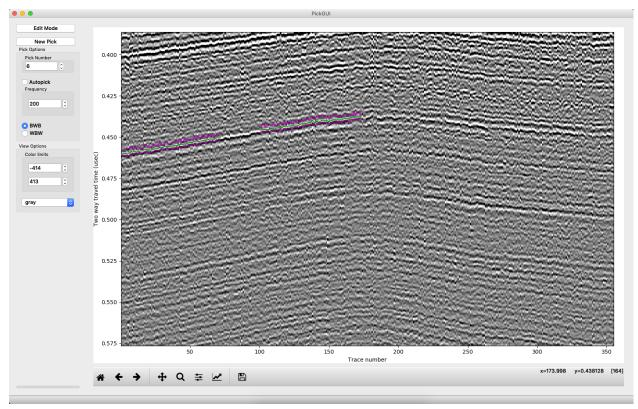
We can also go back and edit a previous pick, moving it up, say. We can also delete picks in the middle of a profile by left clicking at the right edge of the span we are deleting, then right click at the left edge.
