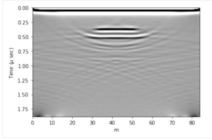
Stolt migration is great in places where the velocity is known to be constant. It is quite a bit faster than the other routines. Here though, we need to be careful about migrating power in from the edges of the domain, as can be seen in the lower corners above. For this reason, we apply a linear taper to the data so that the Fast Fourier Transform being used does not instantaneously switch from data to zeros around the edges.
