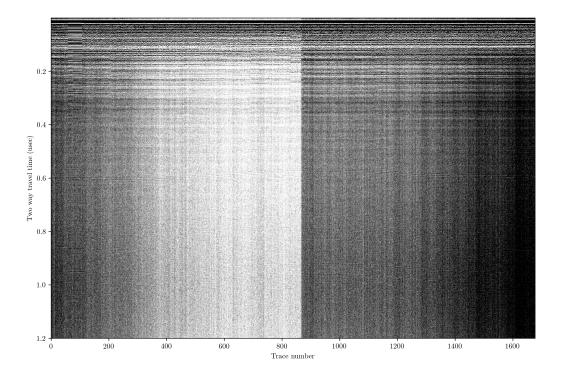
First, lets do some vertical filtering. As before, we will vertically bandpass with a 5th-order forward-backward Butterworth filter from 200 to 600 MHz.
