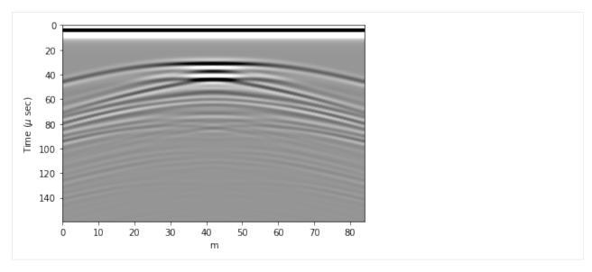
This synthetic image illustrates why we need to migrate. There are large hyperbola that extend away from the actual location of the box in both horizontal directions. These hyperbola, or diffraction curves, do not accurately represent the subsurface stratigraphy, they are only a result of imaging the box from the side as an off-nadir reflector.
